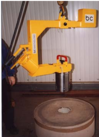
1. Insertion of the gripper into the roll causes its teeth to expand by a built-in self-acting mechanism.
