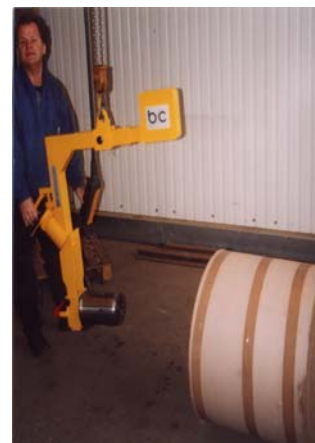
5. .... the gripper can be moved back. The reel feeder is now ready for the next operation cycle.
