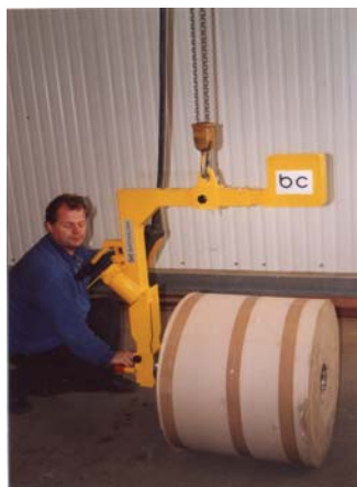
4. On setting the roll down in its horizontal axis position, the hook is furthermore lowered until it is free of the payload. The teeth can now be retracted and ....
