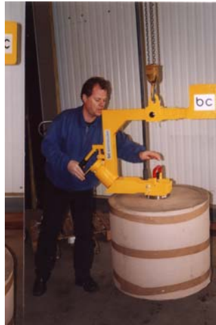
2. After lifting the roll high enough for a carefree turning operation, the operator works the release lever to the right, while he takes hold of the red guide lever with his left hand ...
